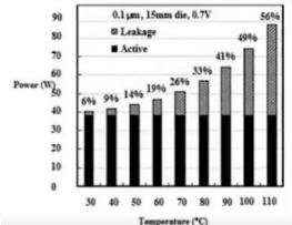
Power Consumption of a die as a function of temperature. Courtesy of Vivek De, Intel.
